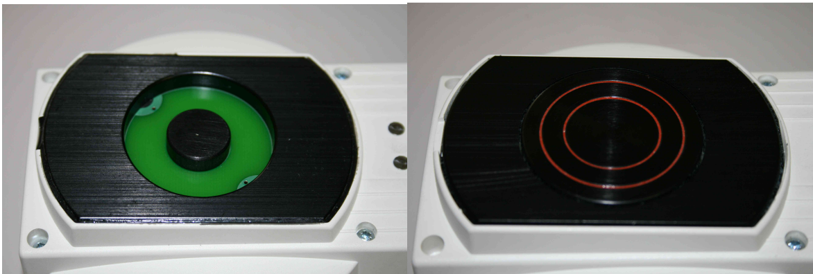
Figure 1. G - type Sensor Electrode Gypsum and Board Products Penetration Depth ~3/4 inch (20mm)
