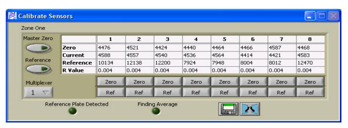
The purpose of the "Calibrate Sensors" screen is to display the raw data and stored values for each Sensor on the IMPS-4400 Sensor array. With no board material running on the line, a manual reset may need to be performed to initialize the IMPS-4400 system by performing a Master Zero upon start-up of the software. Master Zero is always performed when no boards are over the Sensors.
