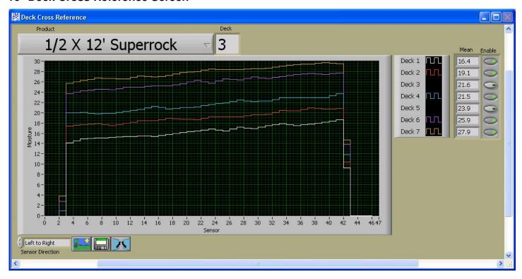
The deck cross reference shows the column moisture average for each deck overlaid on one another. This display is useful for comparing deck performance.
