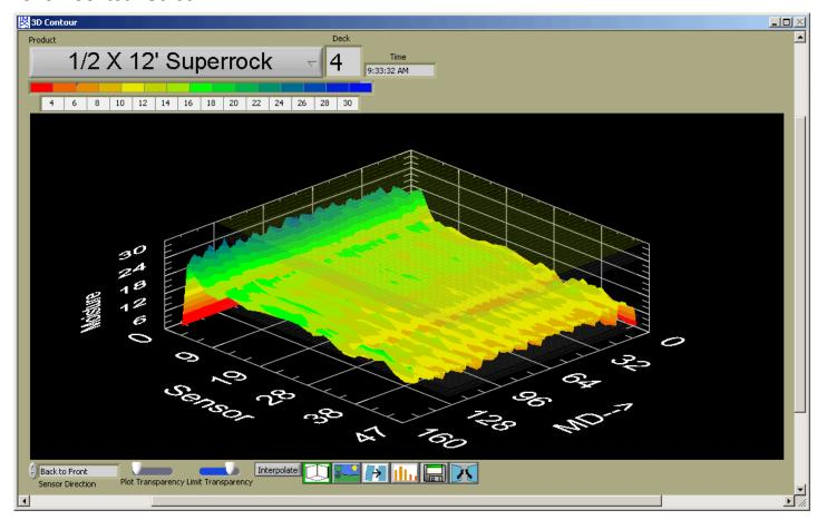
The 3D Contour is similar to the 2D contour with a third axis representing moisture. The high and low alarms and warnings are shown as planes. It can be rotated in any direction to provide any view desired.
