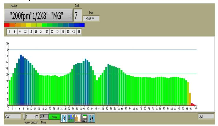
The bar graph shows the column moisture average as each board passes over the Sensors
