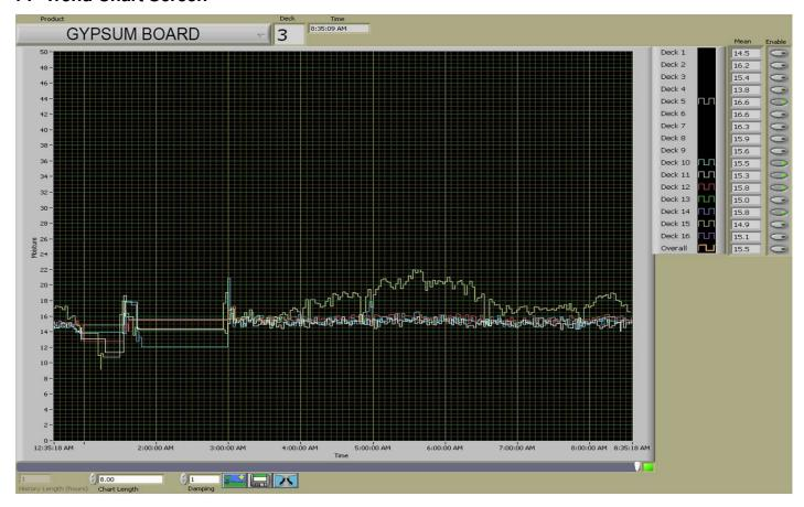
This shows moisture for each deck and average of all decks versus time for each deck and an overall average.
