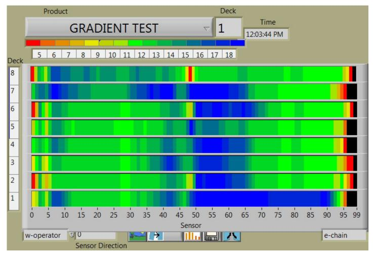
The Multi Deck Display shows the moisture profile of the last boards measured for each Deck.
