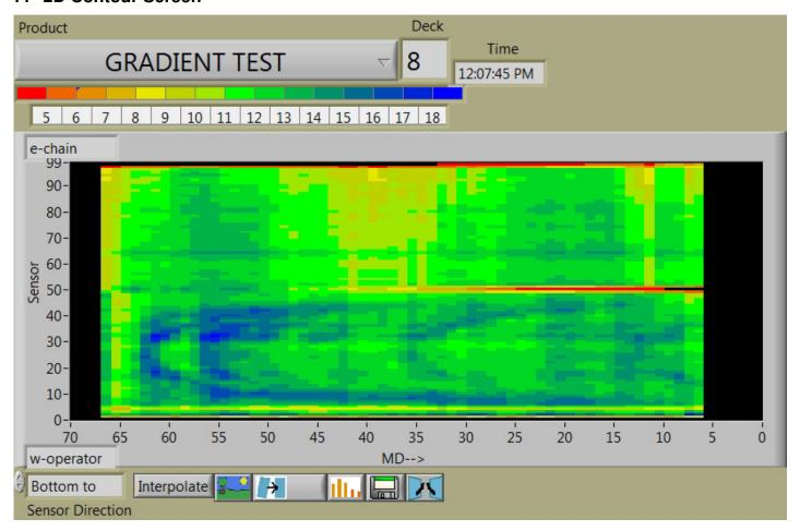
This graph shows a top view snapshot of the boards as they pass over the Sensors. In this example they are traveling from left to right. The Dewander/Deskew, Real Sensors, and Interpolate controls are all tied together between different graph modules. When one of these controls is enabled on any screen, it is enabled on all screens.
